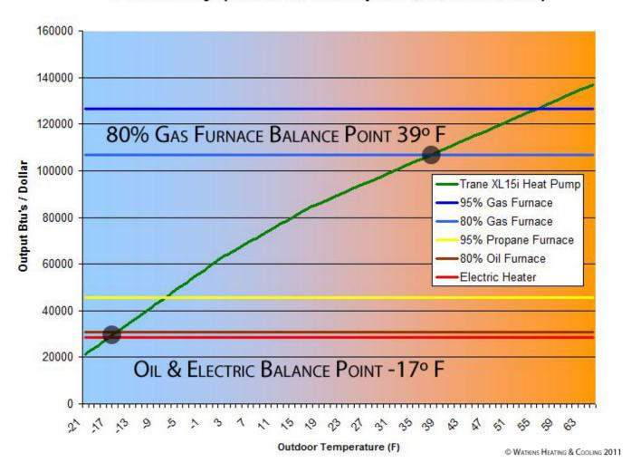
So even though the heat pump is running 24/7 and still can't keep up, the heat that it is producing is still much cheaper than electric resistance heat. The combination of electric heat at 100% efficient and heat pump heat at 300-400% efficient result a total heating system that is more than twice as efficient as electric heat alone. You could also say that adding a heat pump to an electric furnace will cut your heating bills by about 60%.
